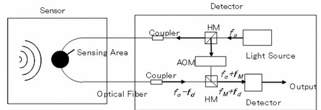
Figure 2. Laser Doppler Interferometer
