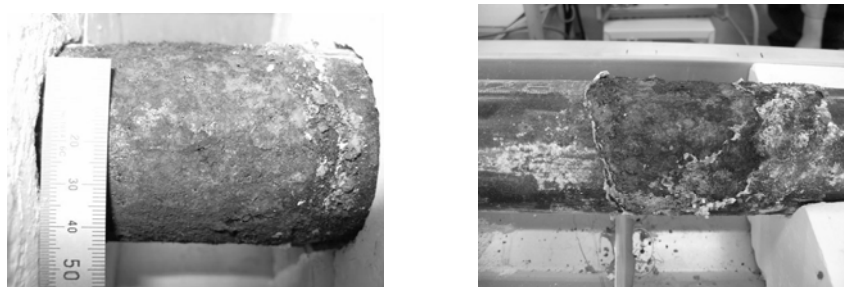
Fig. 7 Corrosion of pipe (left : 1st monitor, right : 3rd monitor)
