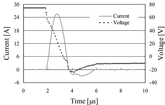
Fig. 4 Typical waveform of the discharge current and voltage
