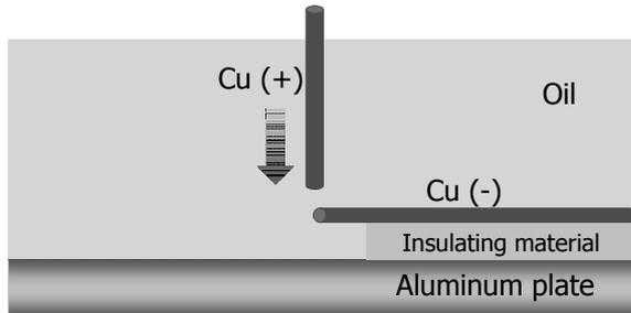
Fig. 6 Model of experimental setup to detect AE wave occurred by cavitations
