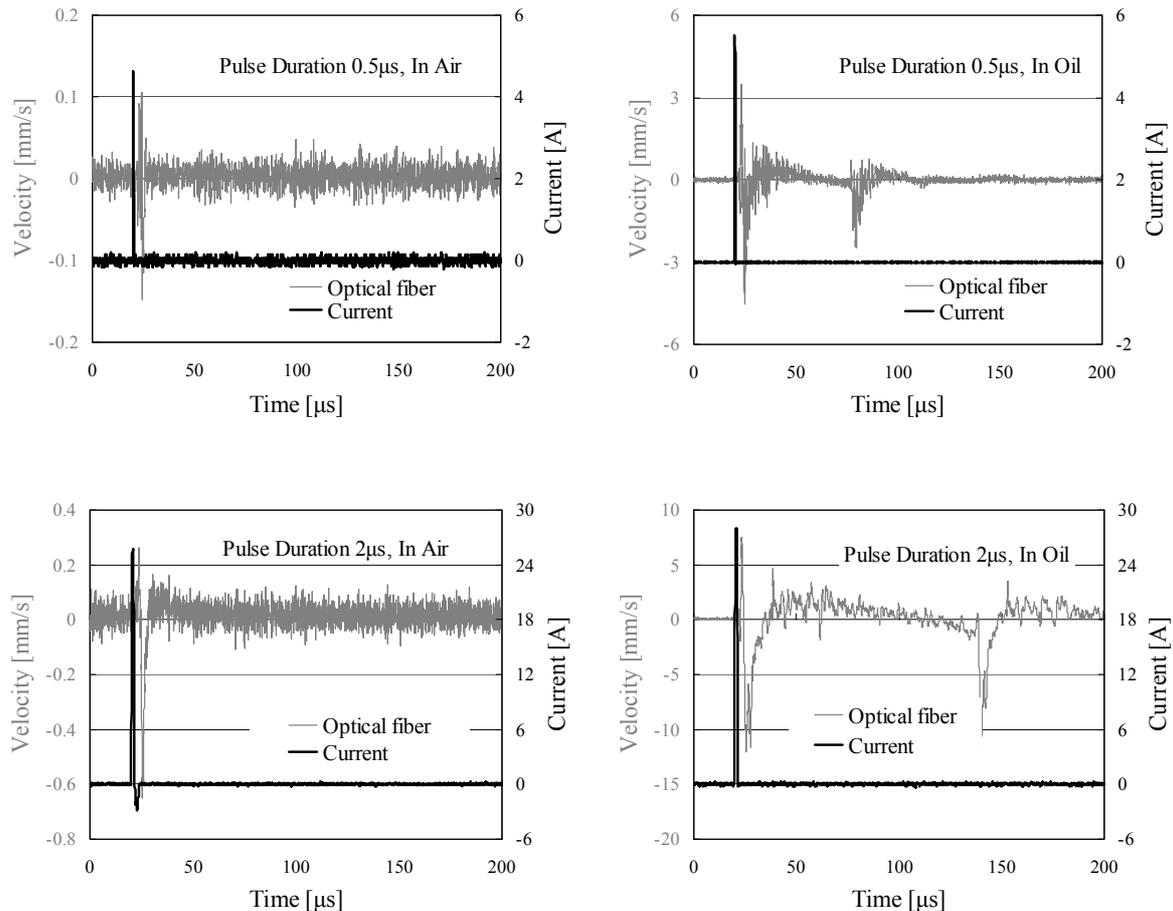
Fig. 5 Detected AE waveforms by optical fiber sensor and current transducer
