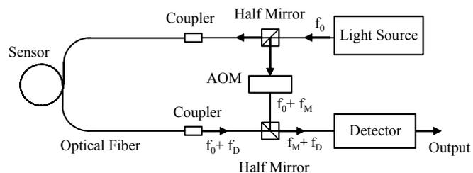
Fig. 1 Schematic view of optical fiber sensor system
