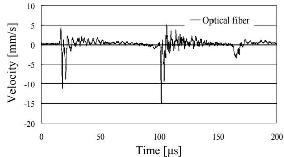
Fig. 7 Detected AE waveforms by optical fiber sensor
