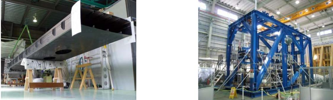
Figure 9. Composite wing box (left) and test equipment (right).
