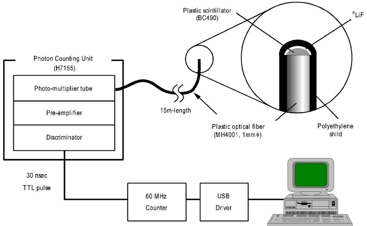
Fig. 1. Schematic diagram of SOF detector system. The SOF detector made up of a small plastic scintillator with  ${}^6\text{LiF}$ , a plastic optical fiber, a photon counting unit and data acquisition system connected to personal computer via USB.
