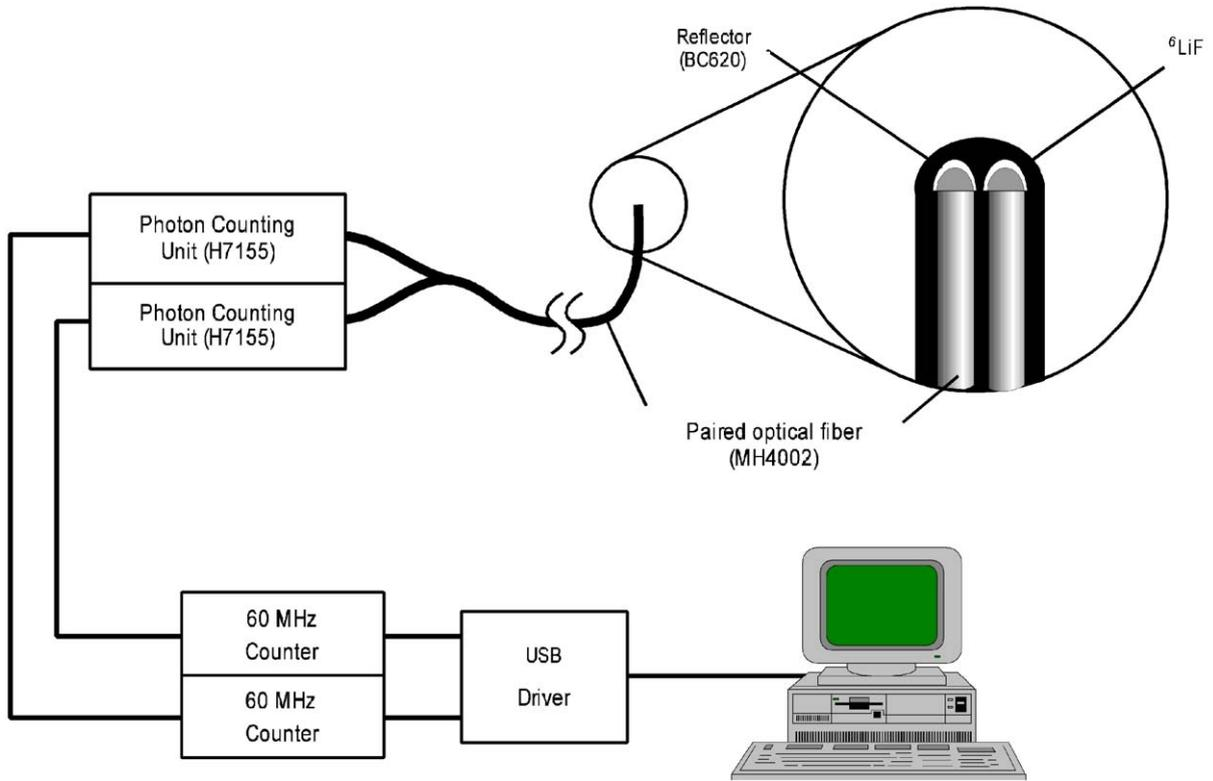
Fig. 5. Schematic diagram of the paired SOF detector system. The signal processing of the paired SOF detector is exactly same as that of a single SOF detector. The paired probe consists of BC490 plastic scintillator with and without  $^6\text{LiF}$ .
