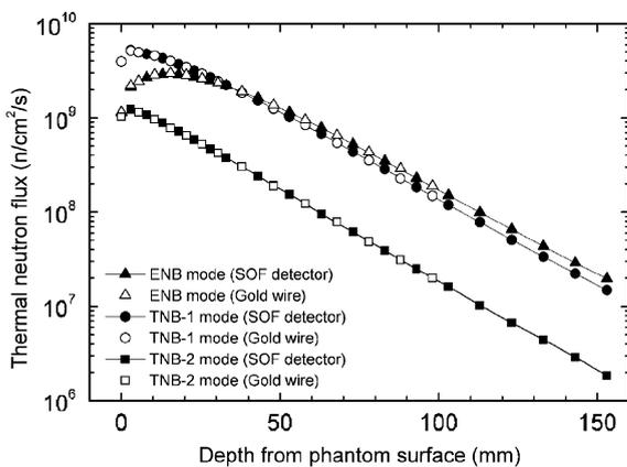
Fig. 10. The measured thermal neutron flux distribution by the paired SOF detector and the gold wire method. The values measured by the gold wire method were corrected in reference to the measured value by the SOF detector at 38 mm.
