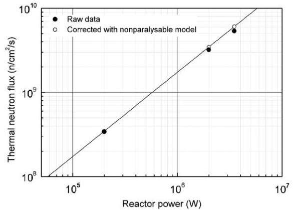
Fig. 9. The linearity experiment data corrected with non-paralyzable system model. A good linearity was observed up to 3.5 MW.
