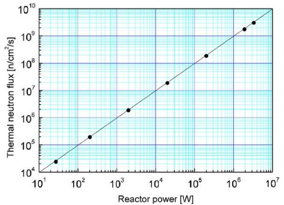
Fig. 7. The result of linearity performance test with paired SOF detector. The compensation effect was observed under 2 kW, and the linearity for the paired SOF detector was guaranteed from 200 W to 200 kW.
