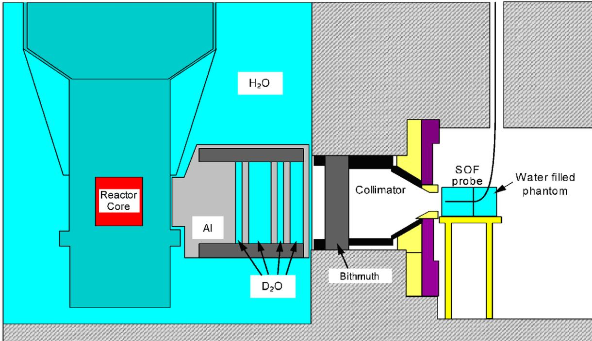
Fig. 2. Experimental setup at JRR-4 medical irradiation facility. The detector probe was placed in an 18.6 cm  $\varnothing$   $\times$  24 cm water-filled phantom whose walls were made from a 3 mm thick polymethylmetacrylate (PMMA) to enhance thermal neutron flux.
