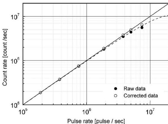
Fig. 8. The pulse counting rate as a function of generated pulse rate. Solid circle and open circle indicate the raw counting rate of SOF detector and the corrected value with non-paralyzable system model, respectively. The dashed line represents the function of the pulse rate with non-paralyzable system model.
