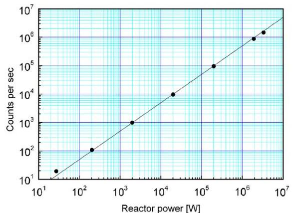
Fig. 3. The measured count rate as a function of the reactor power. Non-linearity was observed under 2 kW and over 200 kW.
