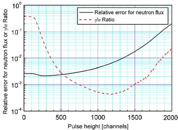
Fig. 6. The relative standard deviation as a function of the discrimination level. The relative standard deviation is minimized at around 300 channels.
