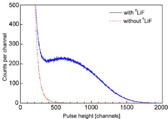
Fig. 4. The pulse height spectrum of a BC490 plastic scintillator with and without <sup>6</sup>LiF neutron converter in a neutron irradiation field. The solid line is the spectrum measured by the BC490 with <sup>6</sup>LiF, and the dashed line is that of without <sup>6</sup>LiF.
